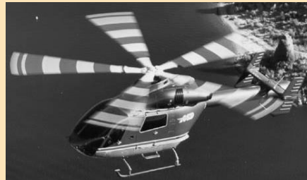
MD900 Explorer: 5-bladed bearingless rotor
