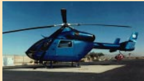
MD900 Explorer: 5-bladed bearingless rotor
